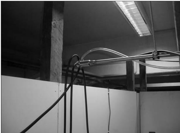
Figure 3 | Distribution of test aerosols via a manifold.
